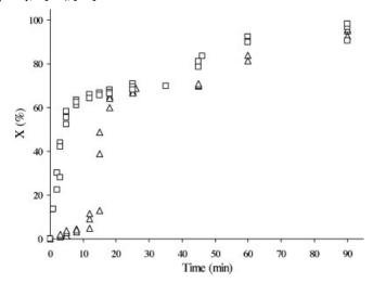
**Figure 1.** Conversion vs. time for the copolymerization at 40 °C of VA/BA/TMI (49/49/2 wt. %) in emulsions stabilized with SDS ( $\Delta$ ) and SDBS ( $\square$ ).
