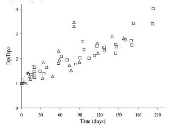
**Figure 4.** Evolution of particle size, during storage at room temperature, with reference to particle size at the end of the polymerization of latexes stabilized with SDS ( $\Delta$ ) and SDBS ( $\square$ ).
