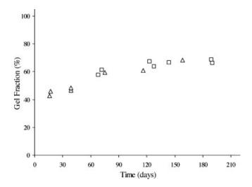
**Figure 5.** Gel fractions as a funtion of storage time of the films cast from latexes stabilized with SDS ( $\Delta$ ) and SDBS ( $\Box$ ).
