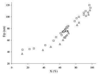
Figure 2. Particle size as a function of conversion for the copolymerization at 40  $^{\circ}$ C of VA/BA/TMI (49/49/2 wt. %) in emulsions stabilized with SDS (Δ) and SDBS ( $\square$ ).
