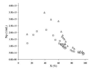
**Figure 3.** Number density of particles vs. conversion for the copolymerization at 40 °C of VA/BA/TMI (49/49/2 wt. %) in emulsions stabilized with SDS ( $\Delta$ ) and SDBS ( $\Box$ ).
